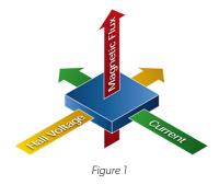
Hall-effect wheel-speed sensors normally provide raw speed accuracy to within 0.5 to 2 percent, and an allowable air gap range of 2 to 3 mm, depending on the target used. These sensors have long met the needs of standard braking systems and offered the flexibility to sense ring magnets or ferromagnetic targets when paired with a back-bias magnet.
